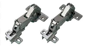
Features & Benefits Heavy duty steel construction, Nickel plated for protection. Spring loaded. 165 degree opening arc.
